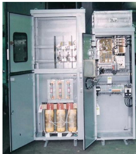
>> Typical "complete" excitation system: 5 KV input LBSF, regulated exciter, solid state application circuit, KinetSync-SR annunciation & logic module, discharge resistors all in a NEMA3R line-up enclosure.
