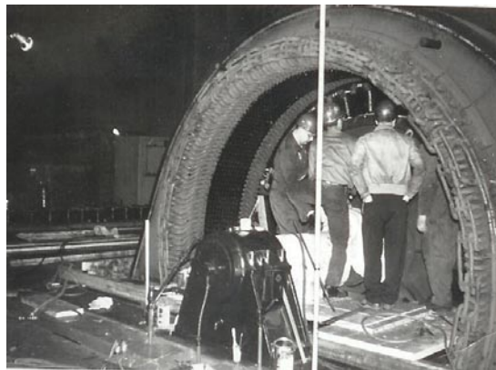
>> Typical large horsepower, steel mill, rolling mill, brush type synchronous motor under repair <<
